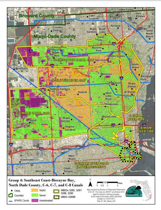
Figure C.1. Distribution of Onsite Sewage Disposal Systems (Septic Tanks) within the Boundaries of WBIDs 3285, 3287, 3288, 3288B, and 3290
